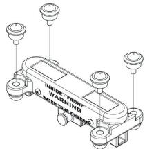
**b)** This is done for both sides, as well as both parts - *Exterior* and *Interior*. In total **4 times**. Note the adjustment holes. Use the holes that get Purgemaster as close to the pipe as possible, but without it touching.
